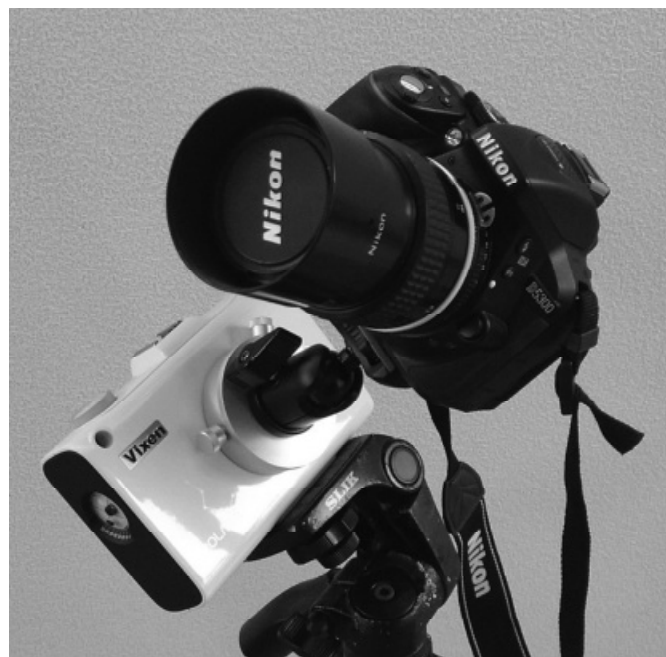
▲ A Nikon D5300 with a 28mm lens mounted on Vixen's Polarie tracker simply with a ball head. The tracker itself sits on a photo tripod with a standard 1/4" screw.
