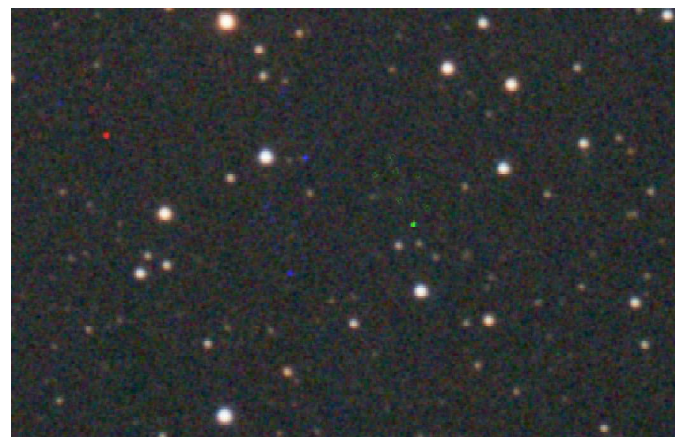
▲ Hot (green, red and blue) sensor pixels can be calibrated away with dark frames.
