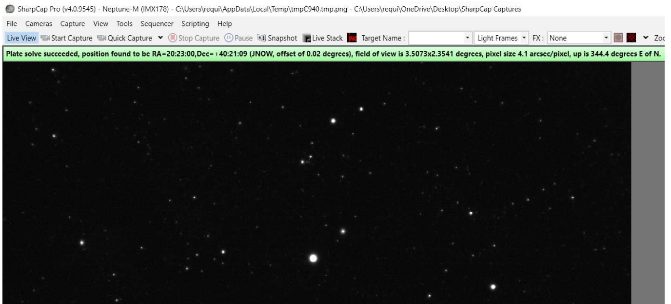
▲ SharpCap 4 Pro screen after successful plate-solving (the bright star is Altair, no histogram stretch applied).
